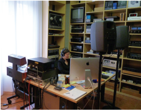
FIGURE 10: Laboratory for the preservation and the restoration of audio documents inside the audiovisual archive of the Fondazione Arena di Verona. On the right, a large collection of recording/replay devices can be observed on the shelves. On the left, an open-reel recorder Studer A812. On the desk, an A/D-D/A Converter PRISM ADA-8XR and two Compact Cassette recorders.
