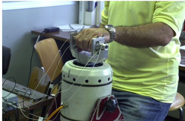
Figure 6. Instrumented handle mounted on the shaker for a dynamic test.
