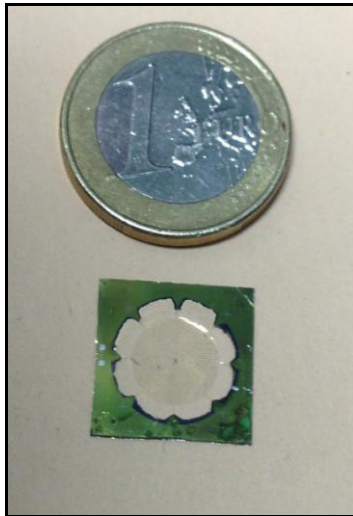
Figure 3. Final spider web bolometer compared with a 1 Euro coin.
