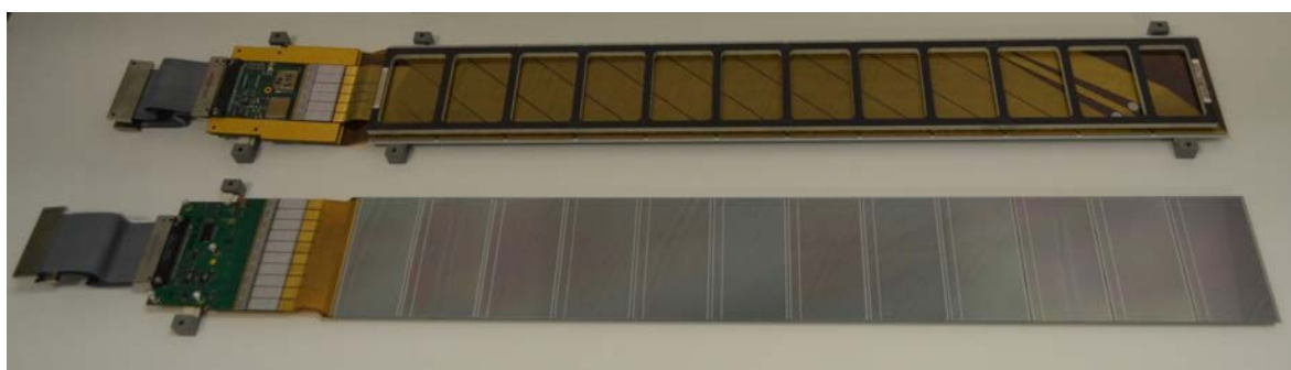
Figure 15. n (top) and p (bottom) sides of a 12 sensors AMS-02 ladder.
