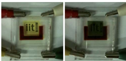
Fig. 5 Images showing the EL5-based PVCC in the bleached (left) and coloured (right) state respectively.
