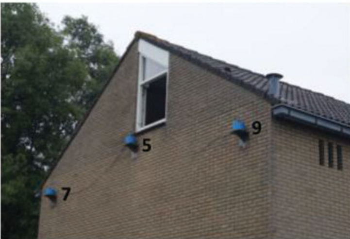
Fig. 4. Geophones applied to a terraced masonry house to measure its frequency characteristics (for this building fundamental periods of vibration of 0.16 and 0.07 s in each direction have been measured) (Eucentre, 2014).
