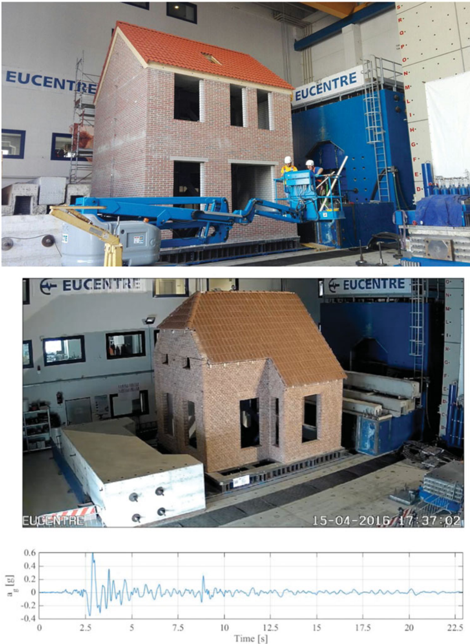
Fig. 6. Two full-scale house specimens on the shaking table (Eucentre, 2015b, 2016b).
