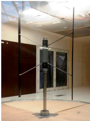
Fig. 4. VAWT model built by the VUB team.
