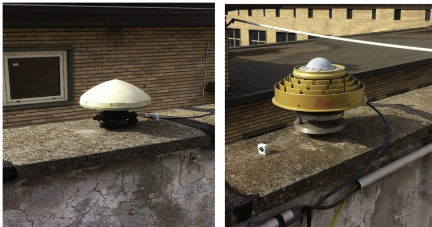
Fig. 4. Rover antenna (right) and master antenna (left).
