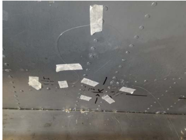
Fig. 6. An example of the FBG sensors installation.
