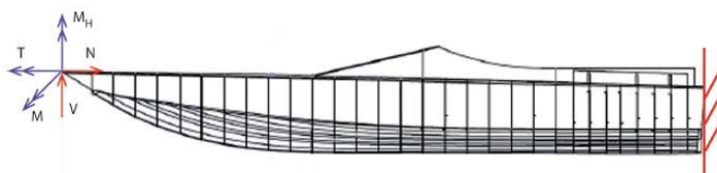
Fig. 8. FE model Loading conditions.
