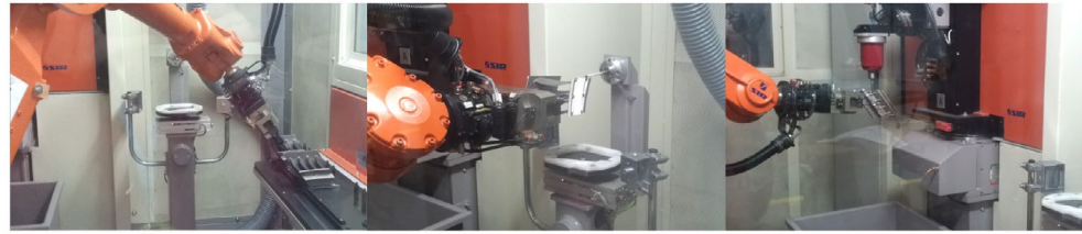
Figure 7. Real robot tasks: component grabbing, surface inspection and deburring.
