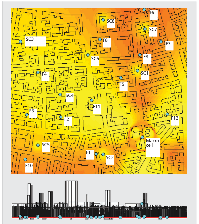
Figure 2. Case study: Map with cell identifiers (SC = micro cell, F = femto cell). Aerial view (top) and side view (bottom).
