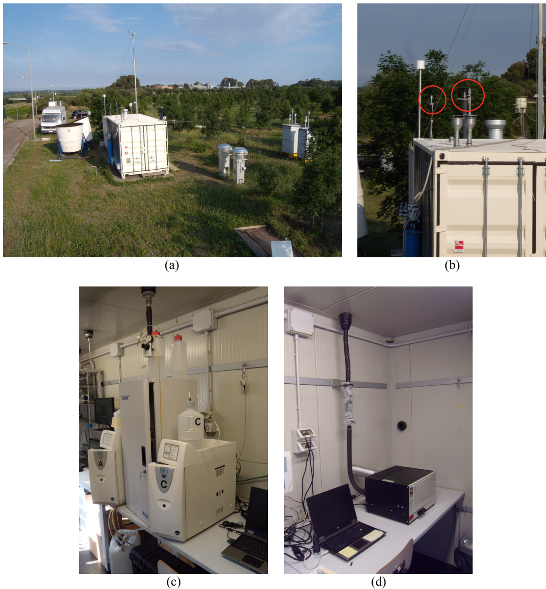
Fig. 1. External view of the trailer and of the reference sampler at the Trisaia site (a), the AIM and Sunset inlets (red circles) located on top of the trailer (b), AIM (c) and Sunset (d) monitors inside the trailer.
