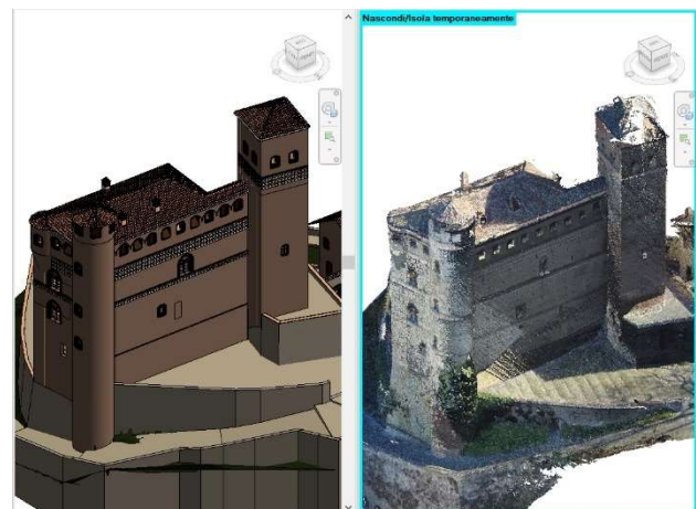
Figure 6. Point cloud usage for supporting modeling stage
