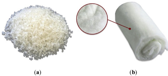
Fig. 4. (a) Polymer grains; (b) Synthetic inert PET wool roll.
