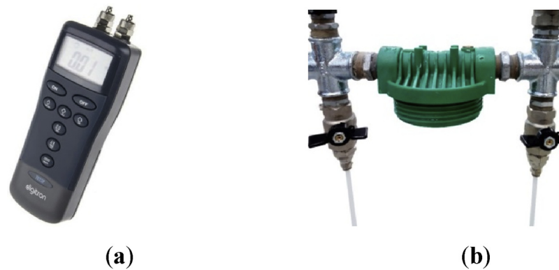
Fig. 7. (a) Electronic differential manometer Digitron 2023 P; (b) derivations along the circuit across the filter for the connection to the manometer.
