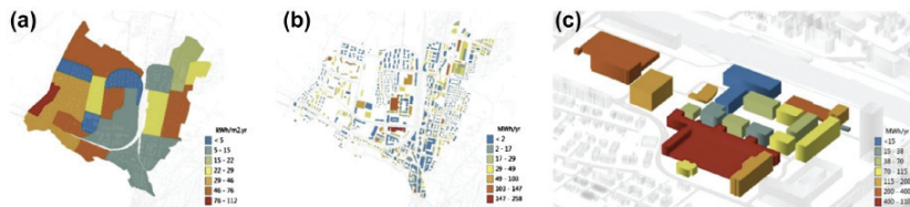
Fig. 5. Energy reduction potential due to retrofit of building envelope, (a) zones in the area of study, (b) buildings in the area of study and (c) buildings in the zone of interest [5]
