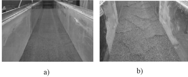
Fig. 2. Sketch of the channel bed configuration: a) flat bed; b) deformed bed
