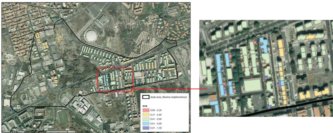
Fig. 1. Map of Nesima Superiore neighbourhood (each building is colored according to its S/V ratio).
