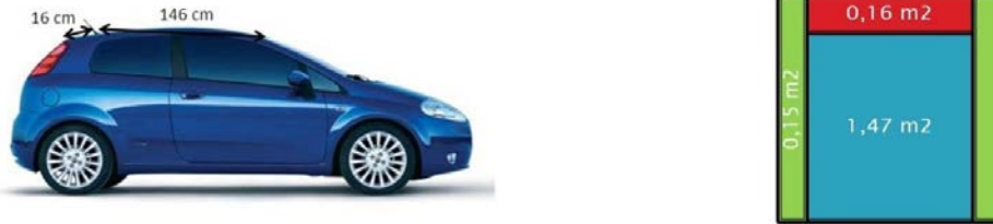
Fig. 8. Roof dimensions of a Fiat Grande Punto
