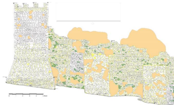
Figure 8. Wall elevation plan on Belvedere Street – Materials: In white the Pietra Forte, in Green the Pietra Alberese, in Yellow the lime mortar, in Light blue the Pietra serena, in Grey the cement mortar, in Orange the Vegetation.
