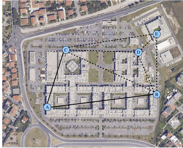
Fig. 4. Connectivity graph of our experimental outdoor mesh network. Solid lines are directional links, while dashed lines are omni-directional links.
