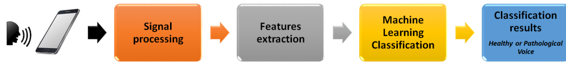
Fig. 1. The flowchart of a possible m-Health system for the voice health state classification.
