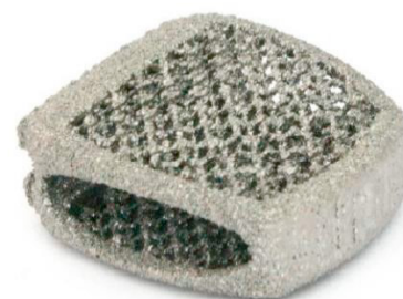
Figure 2c. Modified intervertebral cage in Ti alloy produced by EBM (MC).
