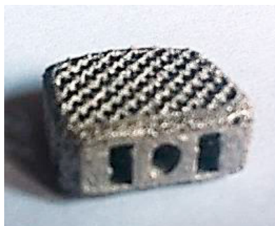
Figure 2b. Intervertebral cage in Ti alloy produced by EBM (SC).
