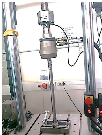
Figure 1b. Compressive setup.
