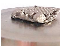
Fig. 5a. Cage SC after the compression test.
