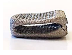
Fig. 5d. Cage 7 after the compression test.
