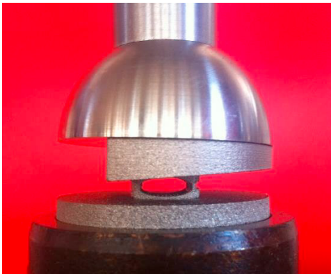
Figure 3a. Cage between the interface blocks.
