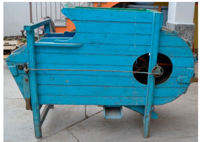
Fig. 12. Traditional cleaner (winnowing) of Piedmont (Italy).
