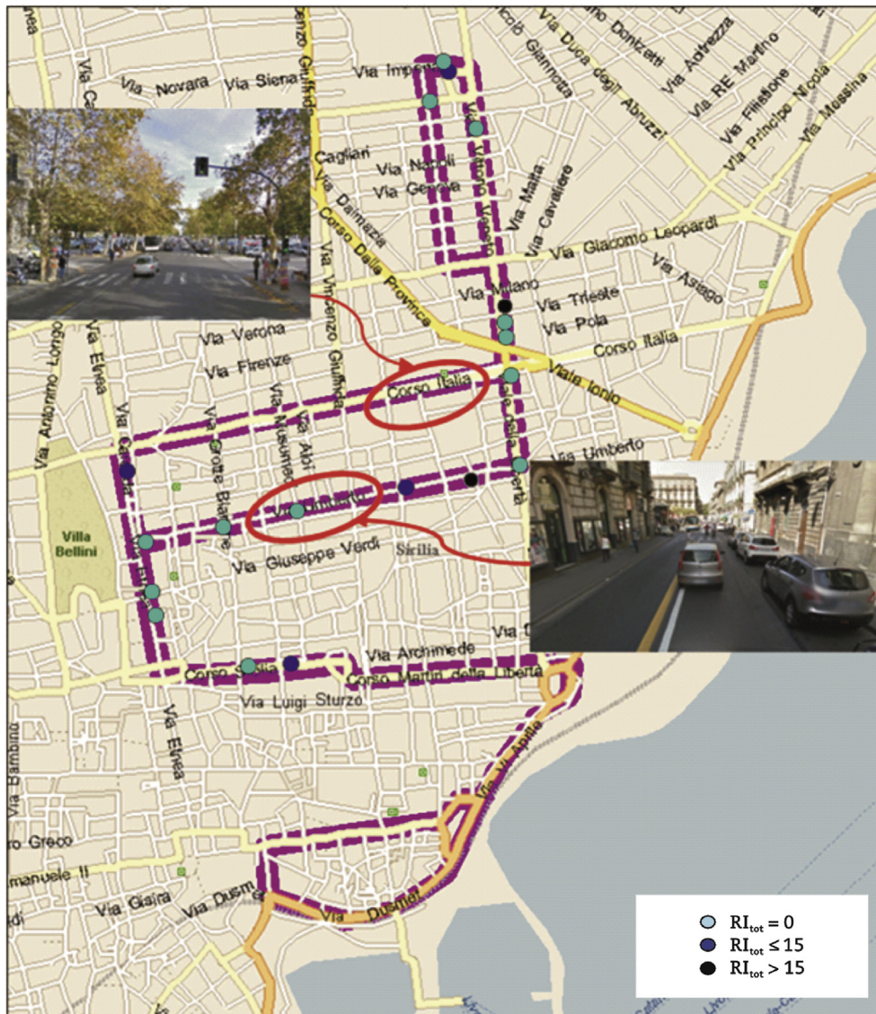
Fig. 7 – Map of traffic conflicts in bus line 2_5 City of Catania, with picture of Corso Italia (top) and via Umberto (down).
