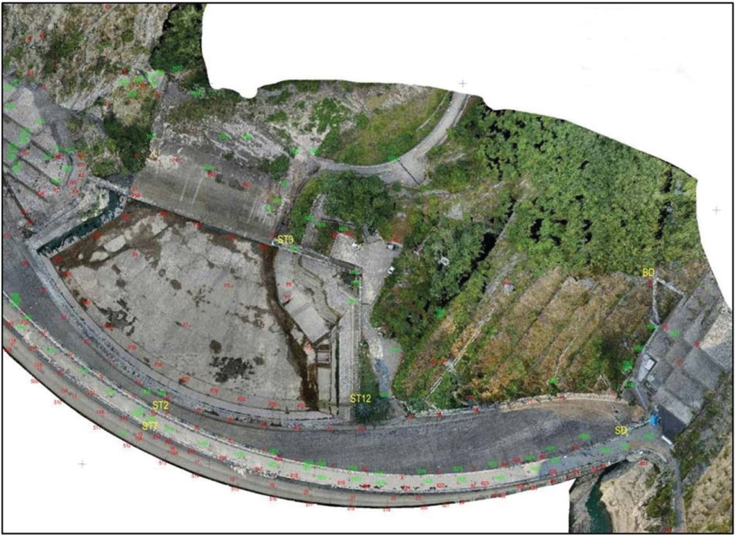
Figure 9. Planimetry of the acquired points (acquired points and laser scanner acquisition bases).
