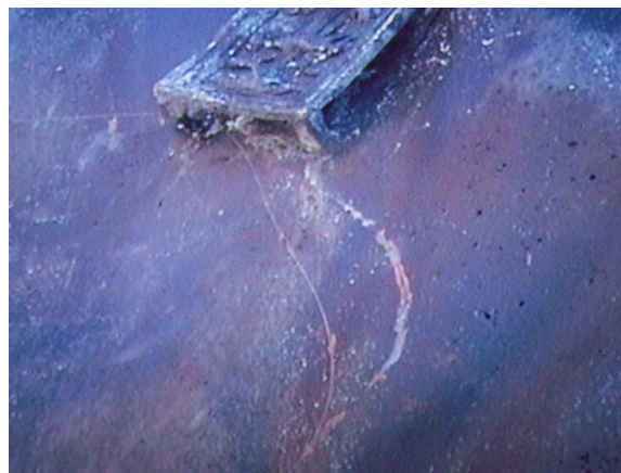
Figure 10: Macrograph showing the sensor detached from the metallic surface.
