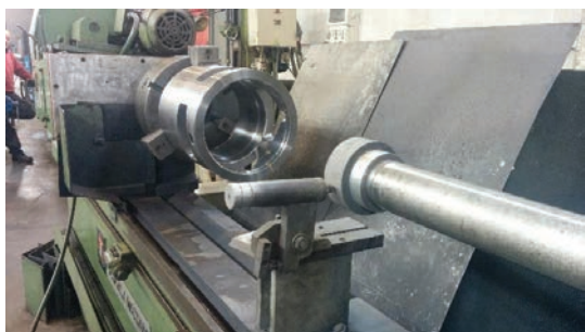
Fig. 2. Dressing operation at Ar.Ter. SrL.
