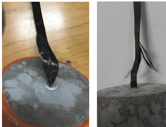
Fig. 4. Failure modes observed in pull-out tests: (a) slippage; (b) fibers breakage.
