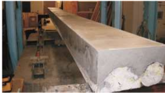
Fig. 13 Beam specimen after concrete curing (LeBorgne, 2007).
