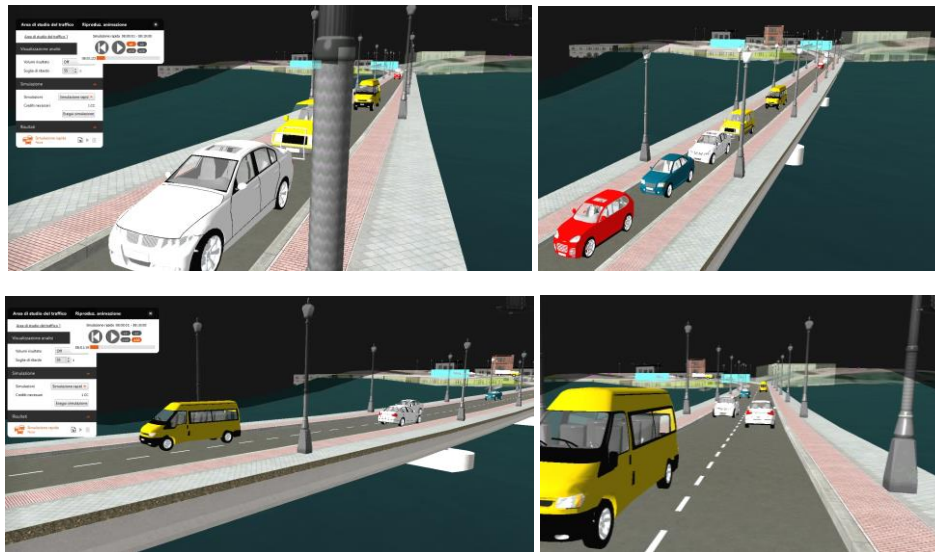
Figure 4. Some images of the traffic simulation in InfraWorks with different lane configurations: a single lane (top) and two lanes (bottom).
