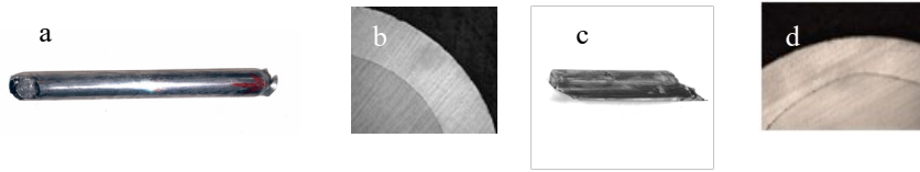
Fig.3. Typical ECAPed specimen; (a) surface quality after one pass; (b) tubular and cylindrical parts after one pass; (c) surface quality after four passes; (d) tubular and cylindrical parts after four passes.
