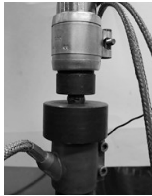
Fig. 2. Upsetting tests configuration and heating strips applied on the forming tools.
