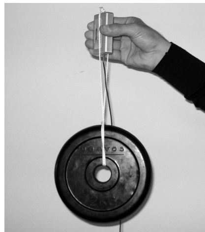
Figure 2. A preliminary experiment had the aim of measuring how grasp force is automatically increased to prevent a grasped object from sliding when the object is pulled down by an external force.
