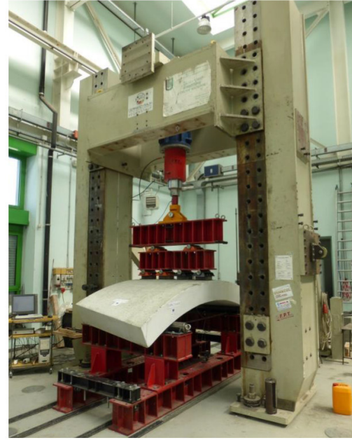
a) b) Figure 5. Bending test: a) front view; b) lateral view.
