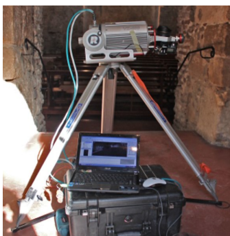
Figure 4. The laser scanner with horizontal inclination of the instrumental axis in the church entrance hall.
