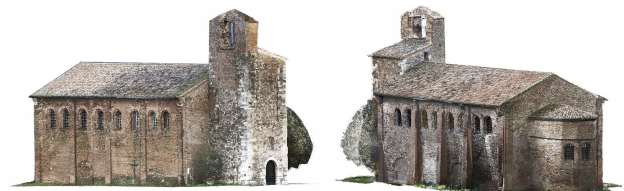
Figure 6. Different views of the final point cloud of the exterior of the church.
