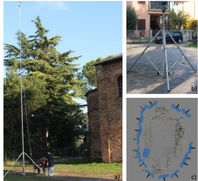
Figure 5. The photogrammetric survey of the church roof; a) and b) equipment used for the images acquisition, c) reconstruction of exterior orientation after the images alignment phase in the SfM processing.
