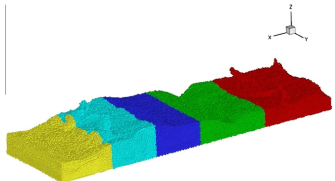
Fig. 2. Example of division of the fluid domain over processors.
