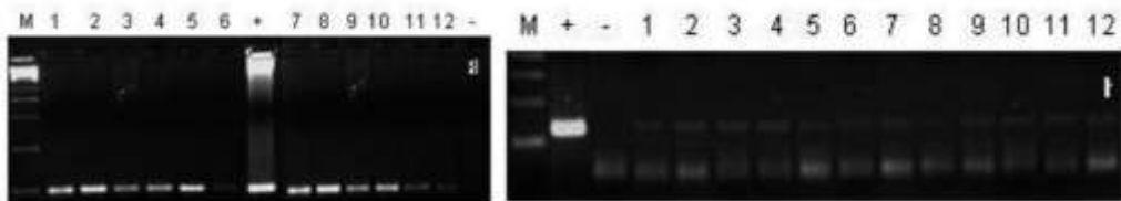
Figure 2. Representative electrophoretic analysis of 35S promoter (a) and CP4 epsps (b) fragments in liver, kidney, heart, muscle, spleen and blood from group T. In each panel, lane M contains a 100-bp DNA ladder, - is a negative control (non DNA template), and + is a positive control (RR soybean meal).
