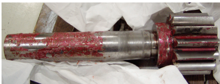
Figure 2: Section of the broken shaft with the pinion still mounted
