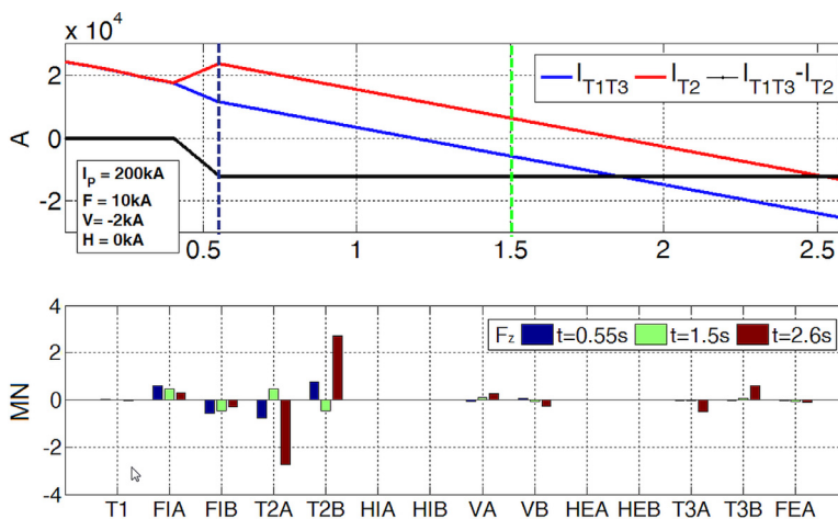
Fig. 7. Vertical forces on the PF coils (on the bottom of the figure) at three typical times of the X-point scenario (shown on the top of the figure).
