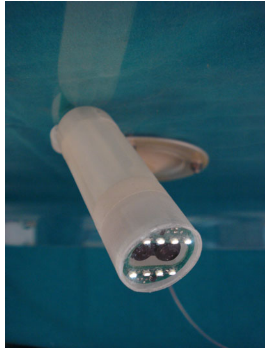
Fig. 7. Assembled prototype magnetically anchored to the abdomen simulator.
