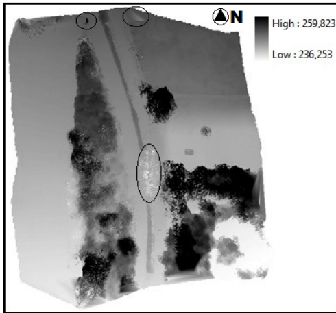
Figure 11. DSM with encircled wrong interpolations (heights in m a.s.l.)
