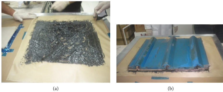
FIGURE 12: (a) Film of resin and (b) placing of the rubber tool.
