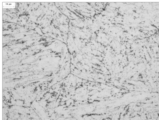
Fig. 5. core microstructure example of nitrided and untreated specimen 500x.
