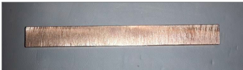
Fig. 1. Squared raw bar (16x16x150mm) for preparation of a specimen.
