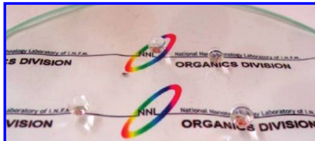
Figure 10. Image of a glass plate coated with a superhydrophobic antireflective bilayer coating.
