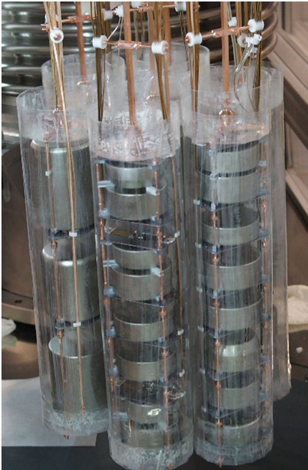
Fig. 31 Photo of GERDA Phase II detector array, showing from left to right string 2 with three semi-coaxial detectors, and strings 3 and 4 with eight BEGe detectors, respectively. Each of the seven strings is enclosed by a transparent mini-shroud
