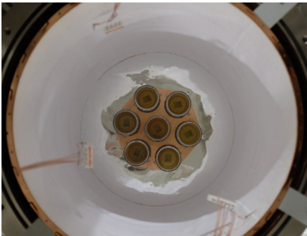
Fig. 11 Bottom PMT plate with 7 PMTs and copper cylinder. Plate and cylinder are covered by wavelength shifting Tetratex® foil soaked in TPB [24]
