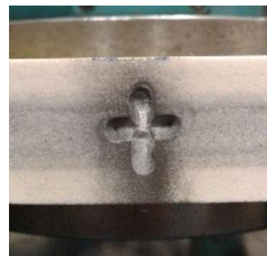
Fig. 2. Damage with shape of “+” inserted on the wheel surface
