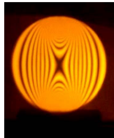
Figure 5. Isochromatic fringes in calibration disk.
