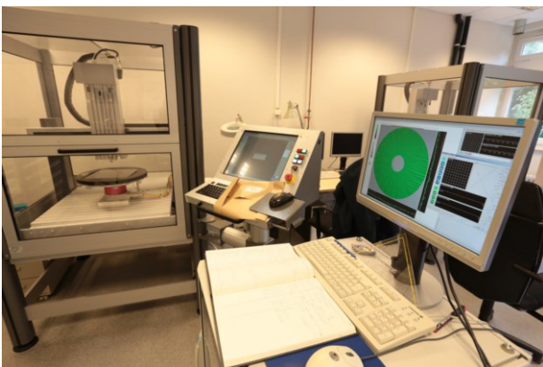
Figure 5. Device for ECS of niobium sheets (scanning head on the left and control computer on the right).
