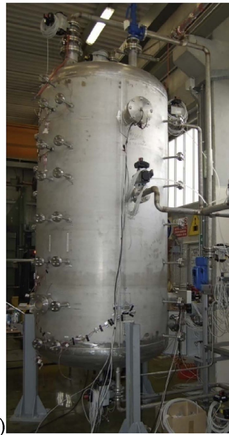
Fig. 3. a, b: CT elevation scheme [7] (a) with indication of the levels and types of sensors (a) and view of the real experimental facility with cold and hot line, components and sensors (b).
