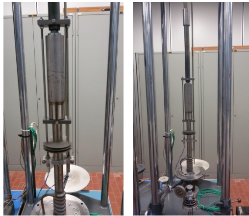
Fig. 2. Cell designed and manufactured for tests in lead, mounted on a MAYES machine.
