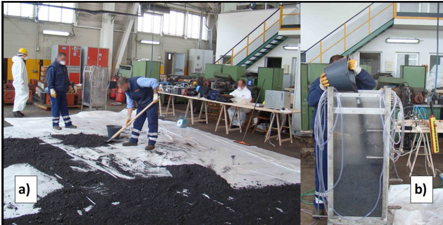
Figure 5: a) View of coal during drying at room temperature; b) phase of prototype filling
