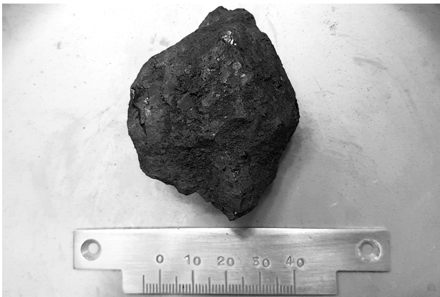
Figure 2: Block of Indonesian Coal subjected to swelling/shrinkage test.
